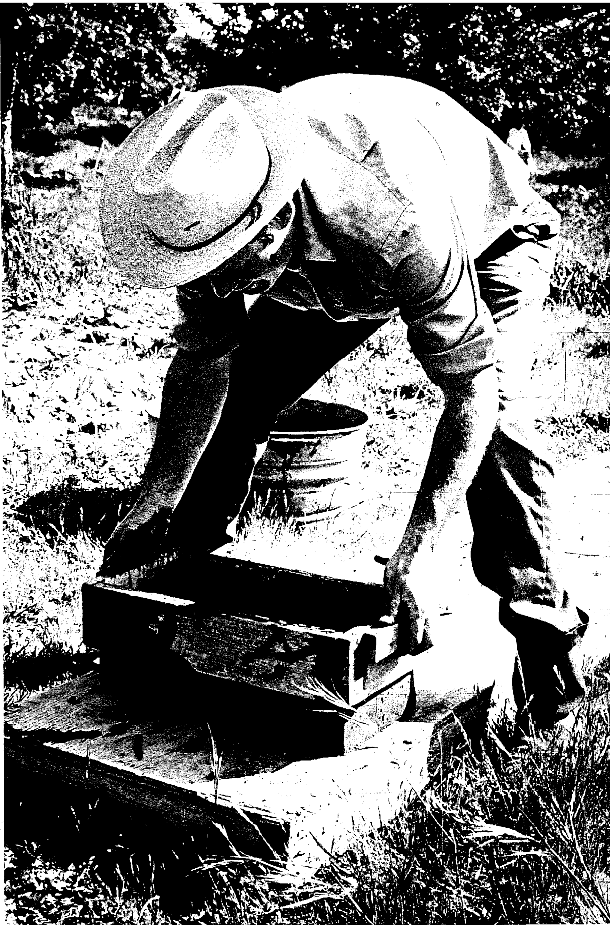
Lifting the mold slowly and evenly to avoid pulling off a corner. If you mixed a good stiff mud, the unsupported wet brick will not sag more than one-quarter inch.
