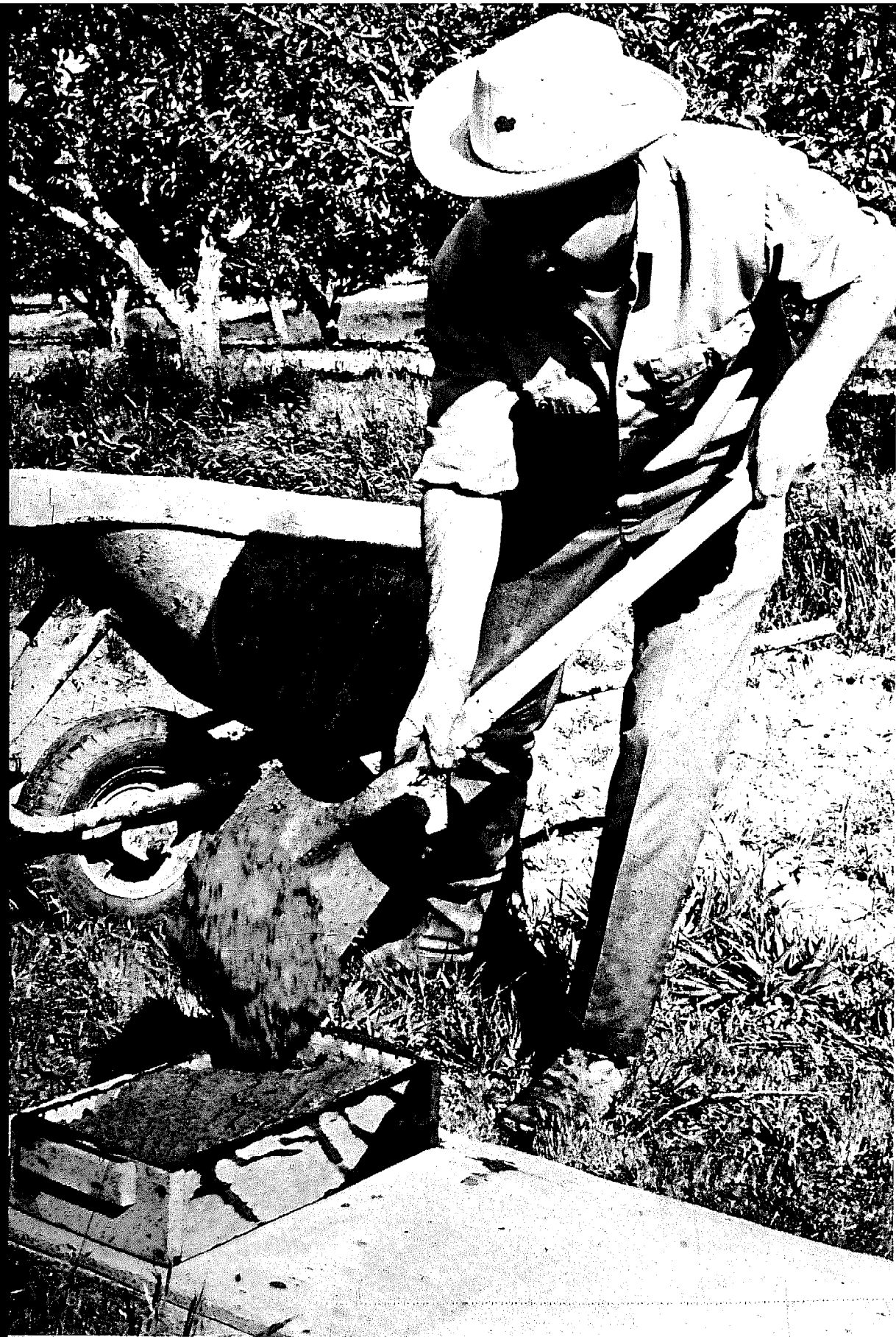
Filling the mold. Note the inside of this mold is lined with tin. The casting surface is made from scrap plywood supported by 2x4's.
